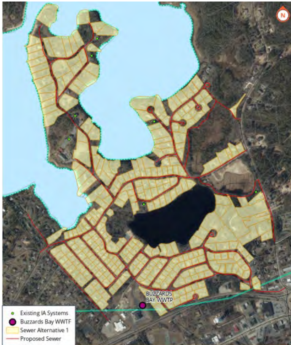
Figure 3: Buttermilk Bay Core Sewer Area - Alternative 1
